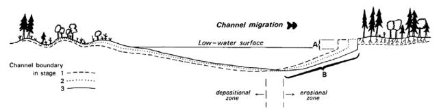
Figure 2. A migrating channel in cross-sectional view. A schematic diagram by Nanson and Hickin (1986) showing a cross-sectional view of a channel at a migrating meander bend. Shifts in the channel through time are indicated by the channel boundary stages and are reflected by the vegetation age progression shown on the depositional (left) side of the channel.
