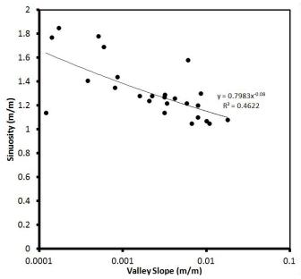
Figure 7. Sinuosity of Puget Sound rivers. alley slope (rise/run) versus sinuosity for major rivers and streams draining to the Puget Sound. Data from Collins and Montgomery (2011).
