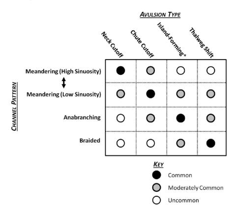
Figure 9. Channel pattern versus predominant avulsion types. The matrix shows unique combinations of different avulsion types occurring within channels of each pattern. Meandering channels are divided into low and high sinuosity types to show the range in avulsion types within. The asterisk indicates that large wood is assumed present so that island-forming avulsions are possible. Thalweg shift describes small-scale avulsions around gravel bars within the active channel (Schumm, 1985).
