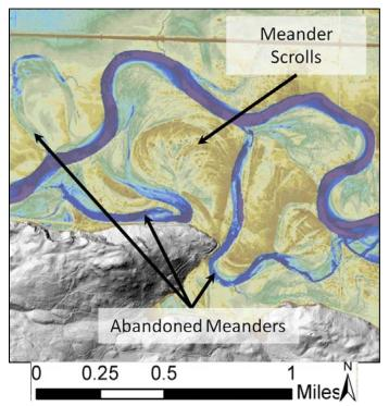
Figure 6. Landforms of a meandering stream. A high-resolution topographic map of the Cowlitz River (Lewis County, WA) floodplain, which is an example of floodplain topography and landforms created by a meandering stream. Multiple abandoned meanders and meander scrolls are visible. The map is colored by relative elevation to the active channel, with cool colors at low elevations relative to the river, and warm colors at high elevations (maximum of 25 feet) relative to the river.
