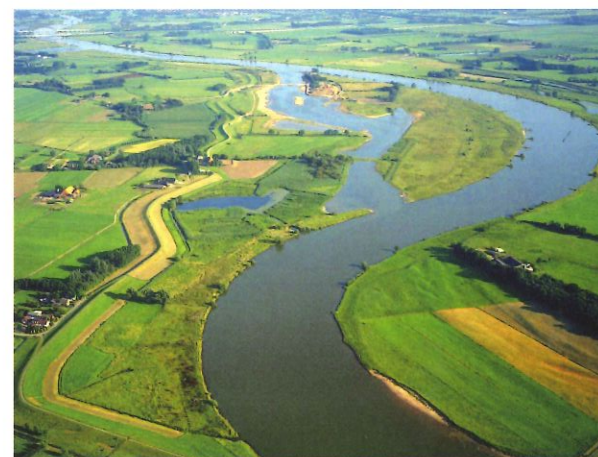
Secondary channel which was dug in the floodplain area along the IJssel River called the Vreugderijkerwaard
