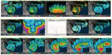
MRMS produces and issues a suite of more than 100 high resolution products over North American on a 1-km grid every 2 to 5 minutes. These data ar used in weather forecast models, and for severe weather, aviation, and hydrometeorology forecasts.
