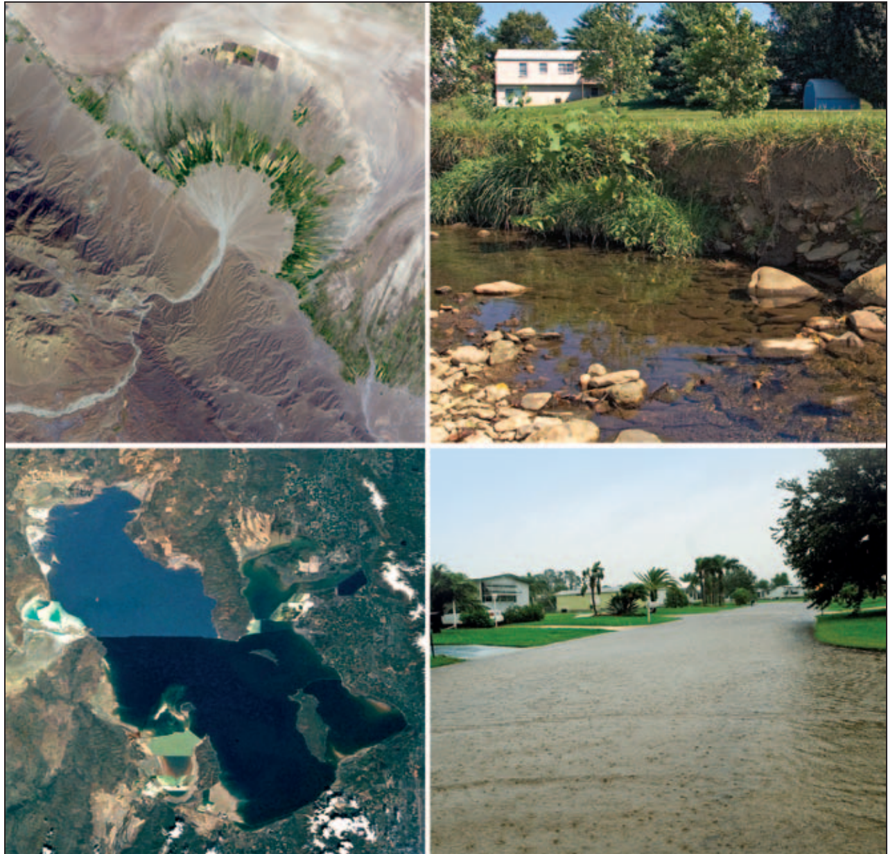
Figure 4-1. Flood-related hazards (top left: alluvial fan; top right: moveable bed stream; bottom left: closed basin lake; bottom right: interior drainage)
